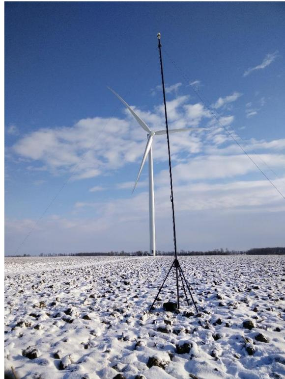
For the duration of the measurement time, acoustic and weather data are logged simultaneously in 10-second intervals. Measurements are conducted when the turbine was operational (Turbine ON) as well as when the turbine was parked (Turbine OFF) in order to quantify the ambient sound level. The microphone board was periodically moved to ensure that all Turbine ON measurements were conducted in a downwind position.
